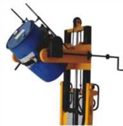
SUITABLE FOR PLASTIC DRUMS WITH 100 MM BELT ADJUSTMENT
